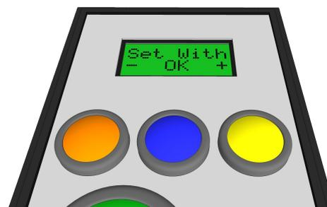
When programming mode is ready the device will display `Select Button`. Press the button for which you wish to set/edit the MIDI command data. The current MIDI command type will be first displayed. To select the type, use the orange (decrease) and yellow (increase) buttons. Once the desired command type is displayed, press the blue (OK) button to accept.
